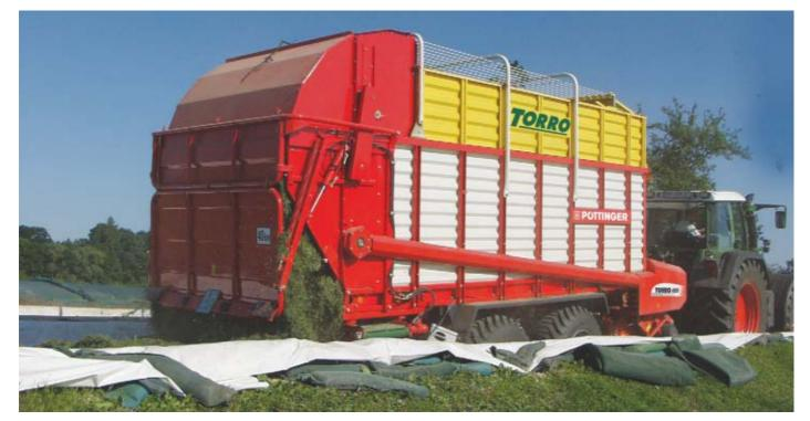
TORRO 4500 5100 45 m<sup>3</sup> 51 m<sup>3</sup> Capacity 28 m³ 31,5 m<sup>3</sup> Volume according to DIN 11741 Pickup width 1,85 m 1,85 m Loading rotor diameter 800 mm 39 Knives max Knife spacing 35 mm Bereifung 500/60-22.5 12 PR Loading area (mm) 5500 x 21006180 x 2100 Width 2550 mm 2550 mm Length (mm L / D) 8414 / 8864 9100 / 9546 Height raised 3970 mm 3970 mm Height lowered 3260 mm 3260 mm 6750 / 7200 6950 / 7400 Weight (kg L / D)
