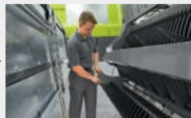
Turn the knives around, and continue with perfectly sharpened knives
