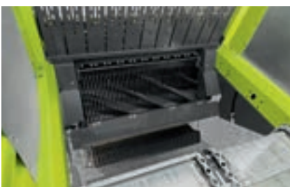
Optimum accessibility with the scraper floor swivelled down by 90°.
