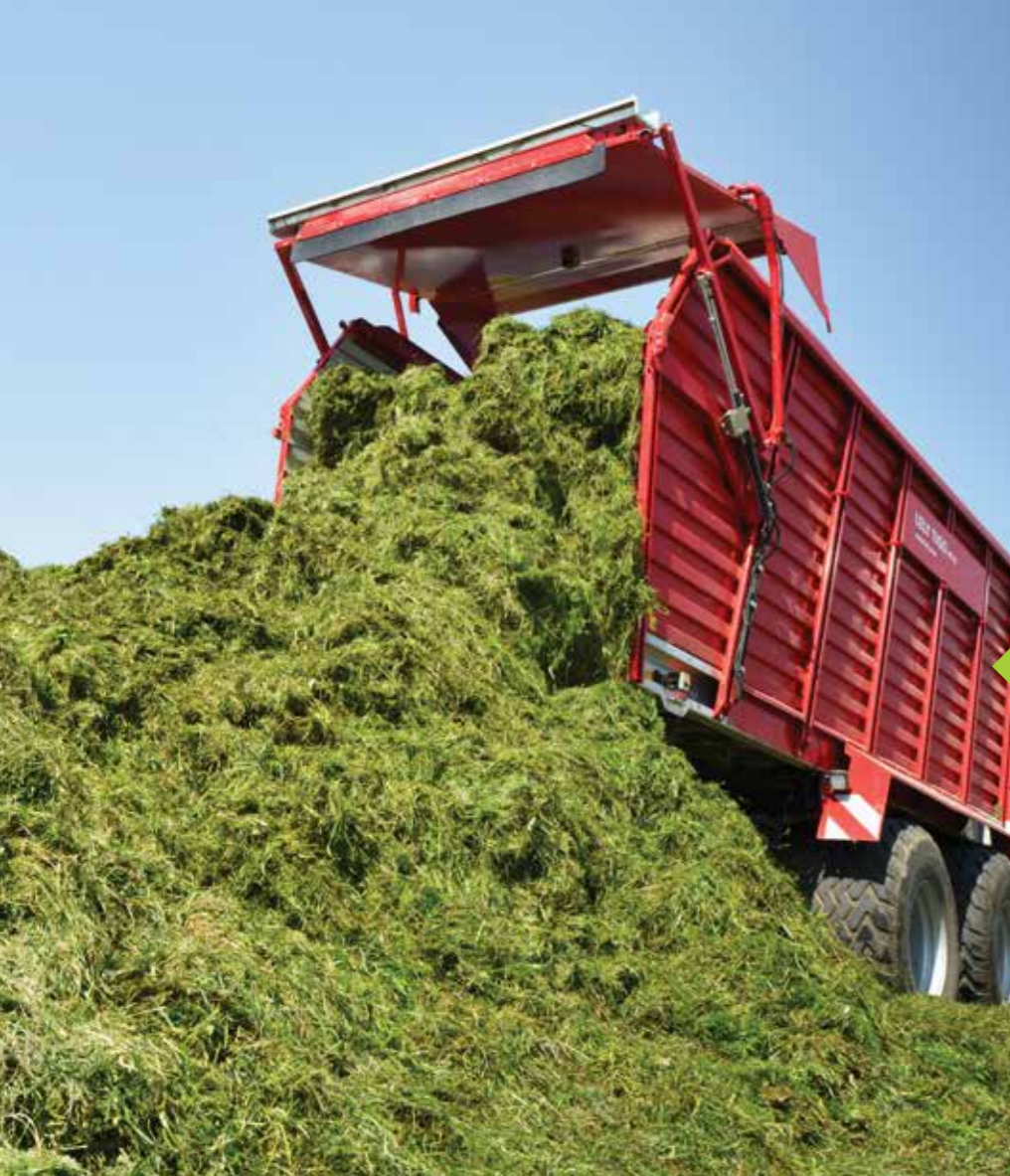
Lely Tigo PR with wide-opening tail gate The tail gate of the Tigo PR with a large opening angle ensures trouble-free unloading, even with large quantities of forage.
